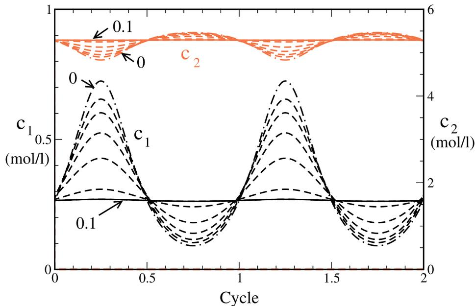
**Figure 3.** The intergranular concentration profiles that correspond to the bulk concentration profiles shown in Figure 2, calculated using an undercooling of  $T_m - T = 20$  K, with  $\Gamma_1 = \Gamma_2 = 3.6$  K/M. Over time, both profiles evolve so that the peak concentrations in the liquid are reduced in amplitude and near-constant levels are attained.
