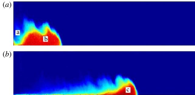
FIGURE 6. The reflected return flow (a) advances along the current until it extinguishes the Kelvin–Helmholtz billow (b) behind the head of the current at the slumping point (c). This mechanism controls the the dynamics of the current but is also an important source of mixing in the head of the current.
