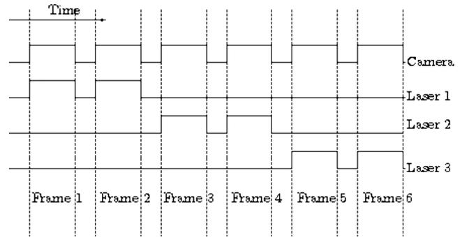
FIG. 2. Timing diagram over 6 frames showing the firing sequence of the camera and three lasers, the full 3D PIV system typically cycles over ten lasers and 20 frames. While this shows three lasers, in principle the system has no limit.
