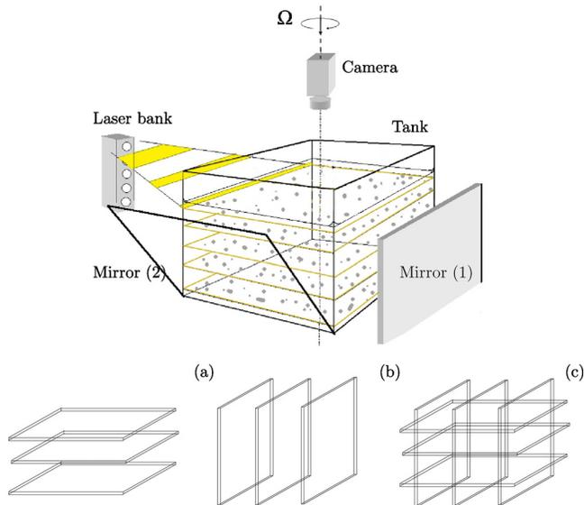
FIG. 1. (Color online) Schematic showing the experimental setup in the top panel and (a) 2D horizontal, (b) 2D vertical, and (c) 3D velocity grids. Mirror (1) is used to amplify the laser intensity and, as described in the text, mirror (2) is used for 3D velocity extraction.
