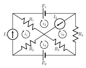
Here the components marked  $E_1$  and  $E_2$  are called *power sources* or *voltage sources*. The components marked  $R_1$ ,  $R_2$ ,  $R_3$  and  $R_4$  are called *resistors*. The components marked  $I_1$  and  $I_2$  are called *current sources*.
