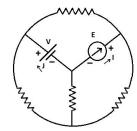
This resistor network has four resistors, each of them having a resistency of 1  $\Omega$ . As usual, we represent the voltage difference across the power source by V and the current across the current source by I. Take the orientation of V, E, I and J as shown in the graph.
